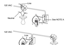
Connect wires "2" and "C" of the TI032-3W to the line (120 V) wire.
